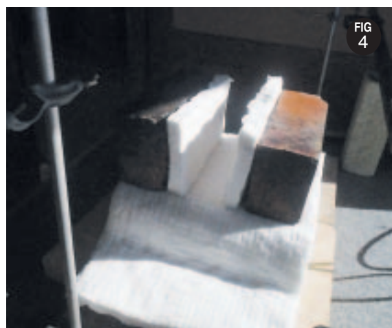
Figure 5: The addition of the ceramic fibre top to the fire box.
