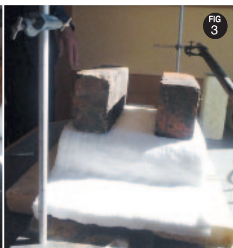
Figure 3: The back of the kiln where the burner will be inserted. Notice the little apron of ceramic fibre wool which forms the base of the fire box and extends out beneath where the burner will be to prevent the heat getting down to the bench.
