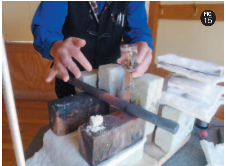
Figure 15: Slaking the thirst of the enlivened quick lime. After the expulsion of the 'dead' gas it has become very lively, giving of great heat, making sounds and moving.
