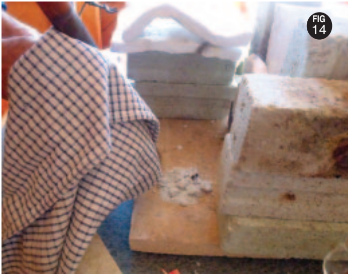
Figure 14: The calcination tube being emptied after 45 minutes. The shiny marble has become chalky white.
